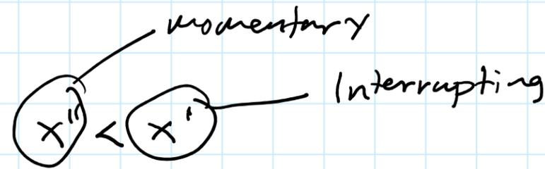
$X'' = 20\% = 0.2 \text{ pu} \rightarrow 1/2 \text{ cycle}$
