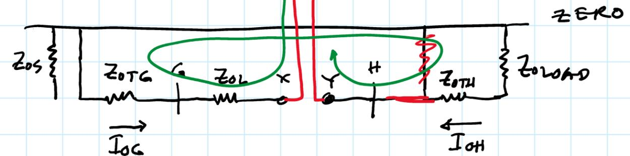
FOR DELTA:  $I_2 = -I_1 \therefore \left| \frac{I_2}{I_1} \right| = 100\%$
