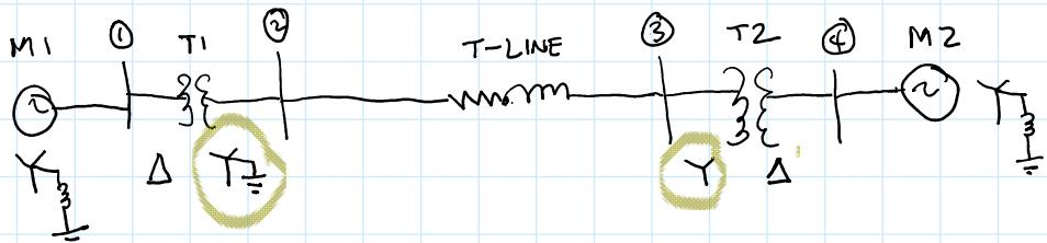
Machines  $M_1$  and  $M_2$  : 100 MVA, 20 kV  $X_d = X_1 = X_2 = 20\%$ ;  $X_o = 4\%$ ;  $X_n = 5\%$
