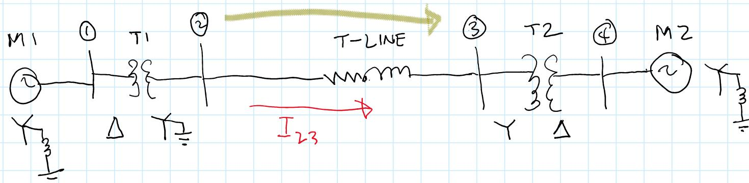
Machines  $M_1$  and  $M_2$ : 100 MVA, 20 kV  $X_d'' = X_1 = X_2 = 20\%$ ;  $X_o = 4\%$ ;  $X_n = 5\%$
